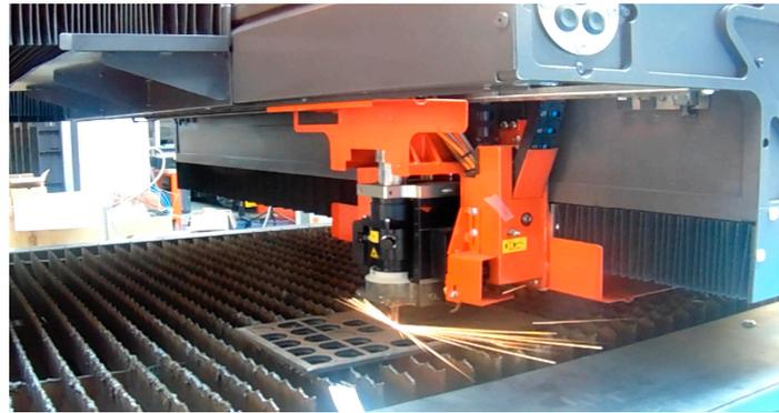
**Figure 1.** Cutting samples with Byspeed 3015 laser installation.
