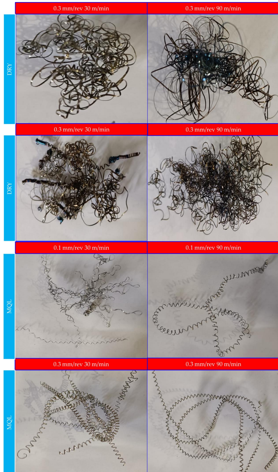
Figure 8. Chip shape variations according to different ratios of cutting conditions.
