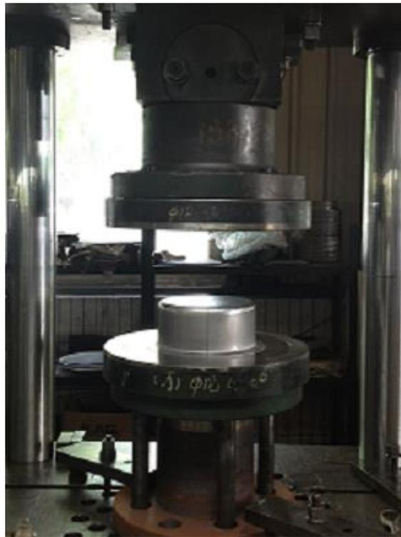
Figure 10. Die assembly for experimental drawing.
