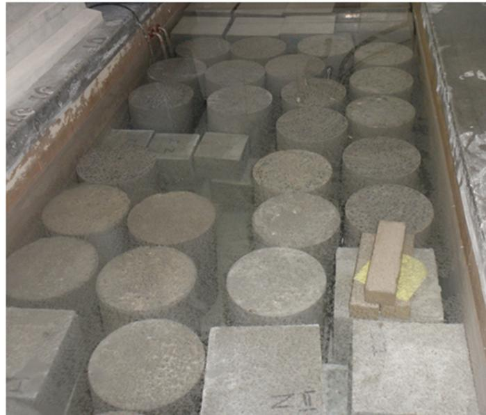
**Figure 2.** Specimens cured for tests in saturated condition.
