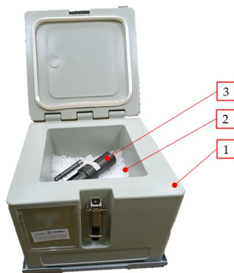
**Figure 5.** Insulated container used to store dry ice powder and condition the experimental setup components, 1—insulated container, 2—dry ice, 3—experimental setup.
