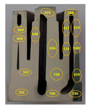
Figure 12. Results of HV microhardness measurements carried out on surface of conformal section of mould core.
