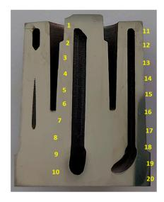
**Figure 9.** Locations of measurement points on surface of core section where chemical composition of SLM 1.2709 steel was determined.
