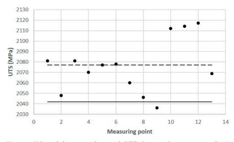
**Figure 16.** Values of ultimate tensile strength (UTS) determined at measurement Points 1 through 13 on cross-sectional area of core (Figure 10) according to DIN SPEC 4864:2019-11: solid line—reference value of UTS = 2042 MPa (determined in static tensile test); dashed line—average value of UTS = 2076 MPa for Points 1 through 13.
