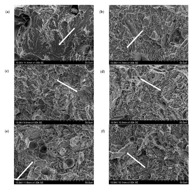
**Figure 7.** SEM images of fractures of circumferentially notched specimens made by SLM method of 1.2709 steel powder after HT490 heat treatment—triaxiality factor values: (**a**) 1.58; (**b**) 0.94; (**c**) 0.73; (**d**) 0.64; (**e**) 0.58; (**f**) 0.51; white arrows indicate areas of brittle fracture.
