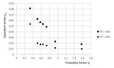
**Figure 6.** Influence of stress triaxiality factor  $\eta$  on equivalent strain  $\varepsilon_{eq}$  of 1.2709 SLM steel subjected to two heat-treatment variants (HT490 and HT540).
