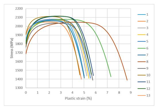
**Figure 11.** Plots of stress–strain function defined at Points 1 through 13 (labelled in Figure 10); test was performed in accordance with DIN SPEC 4864:2019-11 standard.
