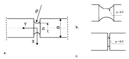
**Figure 1.** Circumferentially notched specimen for tensile tests in triaxial stress state: (a)—letter designation of main dimensions; (b)—notch  $\rho = 6.5$  mm; (c)—notch  $\rho = 0.5$  mm.
