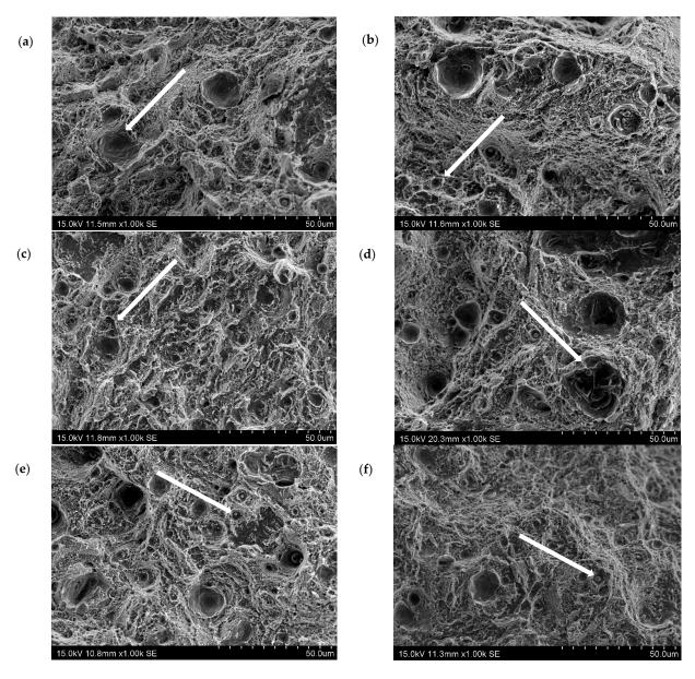
**Figure 8.** SEM images of fractures of circumferentially notched specimens made by SLM method of 1.2709 steel powder after HT540 heat treatment—triaxiality factor values: (**a**) 1.58; (**b**) 0.94; (**c**) 0.73; (**d**) 0.64; (**e**) 0.58; (**f**) 0.51; white arrows indicate where dimple holes are present at the fracture.
