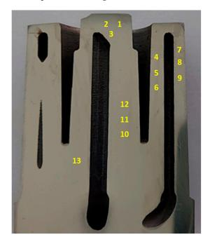
**Figure 10.** Measurement points of yield strength ( $R_{p0.2}$ ,  $R_{p1.0}$ ), ultimate tensile strength (UTS), and plastic strain ( $\varepsilon_{pl}$ ) marked on cross-sectional surface of pressure mould core.
