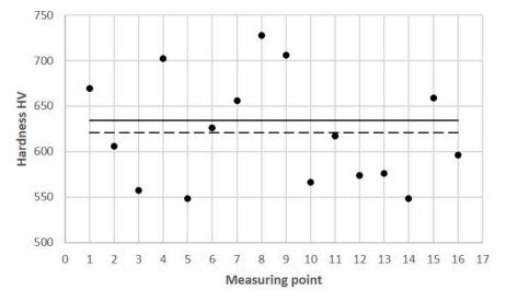
**Figure 18.** Microhardness values determined in 16 measurement areas on cross-sectional surface of mould core (Figure 12): solid line—hardness reference value of HV30 = 636 (determined on printed samples); dashed line—average microhardness value of 621 HV in 16 measurement areas.
