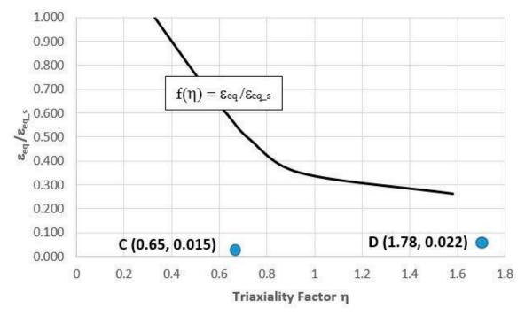
**Figure 14.** Locations of Points C and D with coordinates defined by strain quotient  $\varepsilon_{eq}/\varepsilon_{eq_s}$  and value of triaxiality factor  $\eta$  determined by FEM method during one cycle of pressure machine against experimentally determined function  $f(\eta) = \varepsilon_{eq_s}$  for SLM steel after HT540 heat treatment: Point C—value of function in vicinity of rectilinear channel; Point D—value of function in vicinity of channel with curvilinear axis trajectory.
