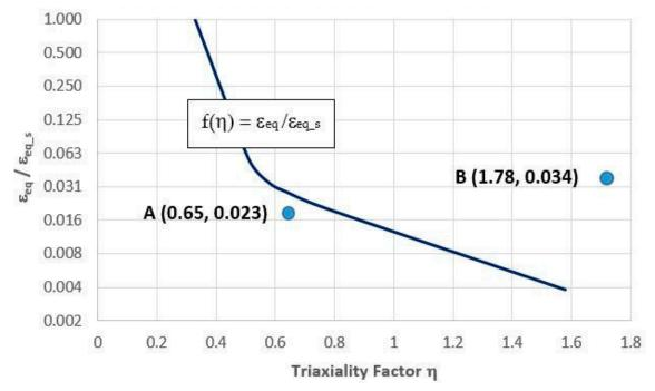
**Figure 13.** Locations of Points A and B with coordinates defined by strain quotient  $\varepsilon_{eq}/\varepsilon_{eq_s}$  and value of triaxiality factor  $\eta$  determined by FEM method during one cycle of pressure machine against experimentally determined function  $f(\eta) = \varepsilon_{eq_s}$  for SLM steel after HT490 heat treatment: Point A—value of function in vicinity of rectilinear channel; Point B—value of function in vicinity of channel with curvilinear axis trajectory.
