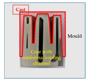
Figure 2. Position of mould core, mould, and casting in geometrical model.
