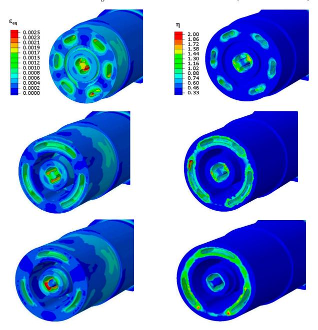
**Figure 3.** Field values of equivalent strain  $\varepsilon_{eq}$  (**left** column) and triaxiality factor  $\eta$  (**right** column) shown in three cross sections of core with conformal cooling channel approximately two seconds after metal was injected into mould.
