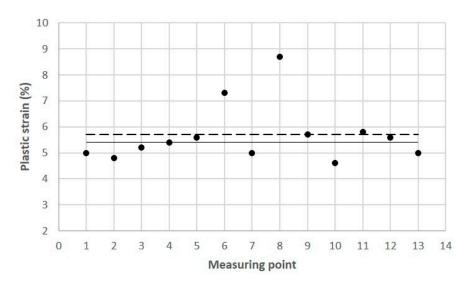
**Figure 17.** Plastic strain values ( $\varepsilon_{pl}$ ) determined at Measurement Points 1 through 13 on crosssectional area of core (Figure 10) according to DIN SPEC 4864:2019-11: solid line–reference plastic strain value  $\varepsilon_{pl} = 5.41\%$  (determined in static tensile test); dashed line–average value of  $\varepsilon_{pl} = 5.70\%$ for Points 1 through 13.
