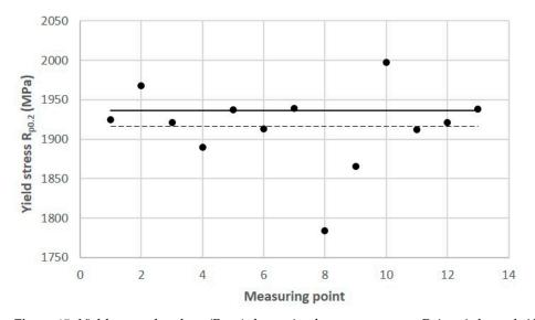
**Figure 15.** Yield strength values ( $R_{p0,2}$ ) determined at measurement Points 1 through 13 on crosssectional area of mould core (Figure 10) according to DIN SPEC 4864:2019-11: solid line—reference yield strength value  $R_{p0,2} = 1936$  MPa (determined in static tensile test); dashed line—average value of  $R_{p0,2} = 1916$  MPa for Points 1 through 13.
