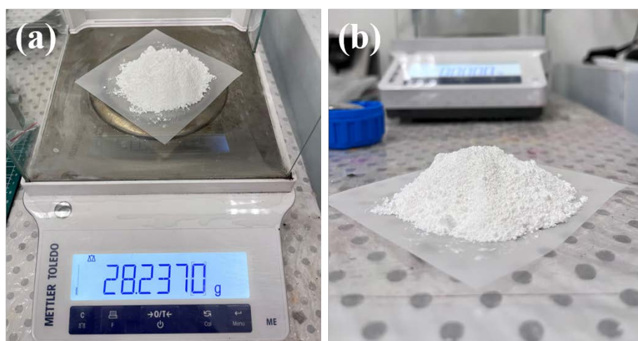
Figure S11. Photographs of (a) about 28 g of BT-190 product and (b) BT powders.
