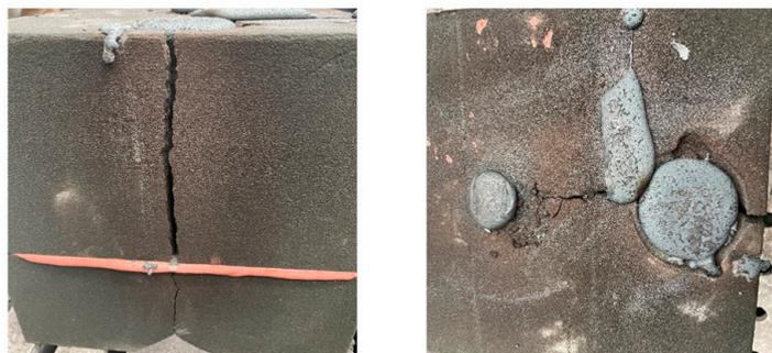
**Figure 16.** Cracks on the sand mold.
