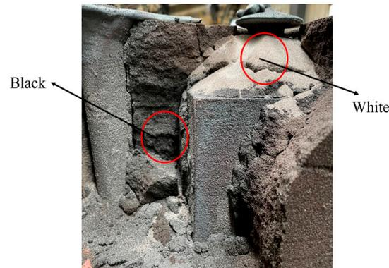
**Figure 14.** Resin sand burnout situation.
