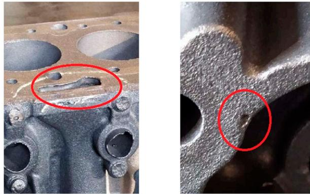
**Figure 1.** The location of the porosity defects in the engine cylinder block.
