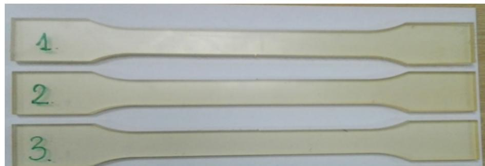
**Figure 4.** Elastomeric samples for uniaxial tensile test.
