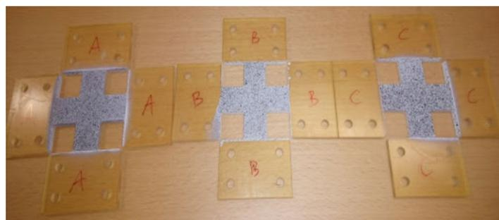
**Figure 7.** Elastomer samples prepared for the biaxial tensile test.
