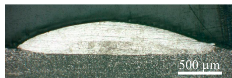
Figure 20. The morphology of the cross-section of the track with optimal process parameters.
