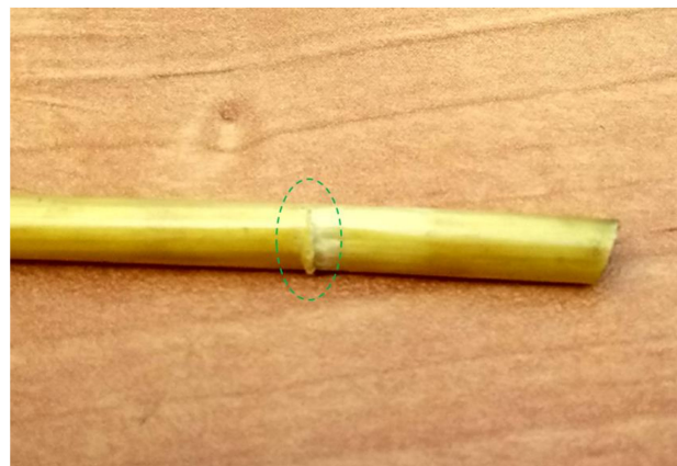
Figure 9. General view of a partially cut straw stem from a test attempt with an offset value g = 0.2 mm.
