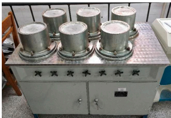
Figure 8. Samples installed on the impermeability instrument.
