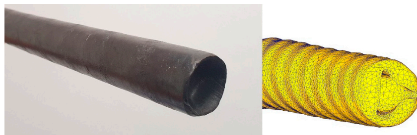
Figure 8. Comparison of the shape change of the rolled experimental bar with the previously obtained FEM model.
