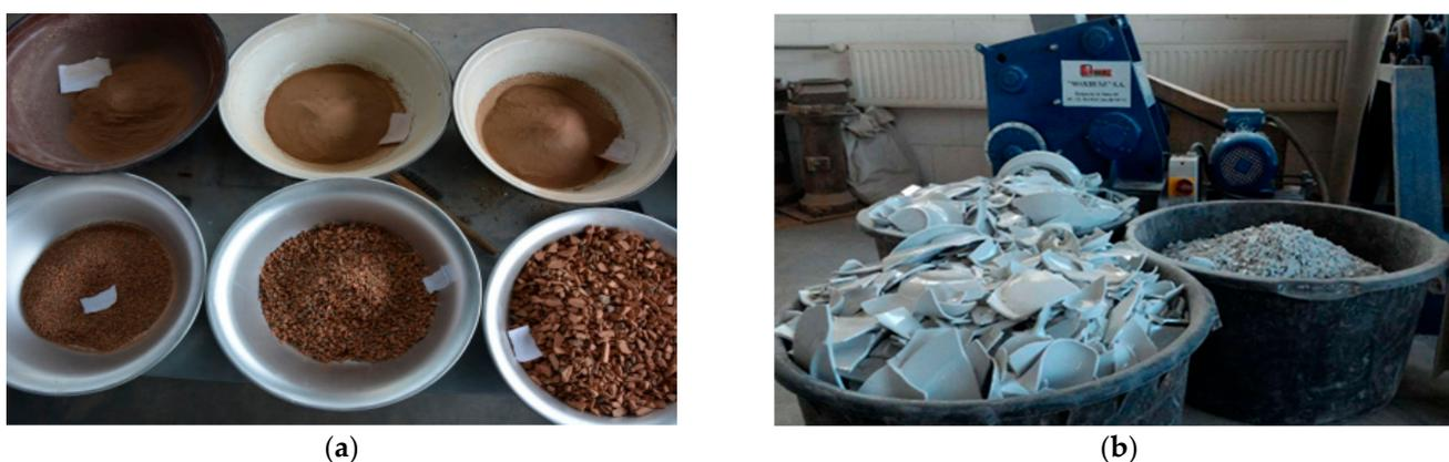
**Figure 1.** (a) Red ceramic waste after crushing and sieving. (b) White ceramic waste during crushing in jaw-crusher.
