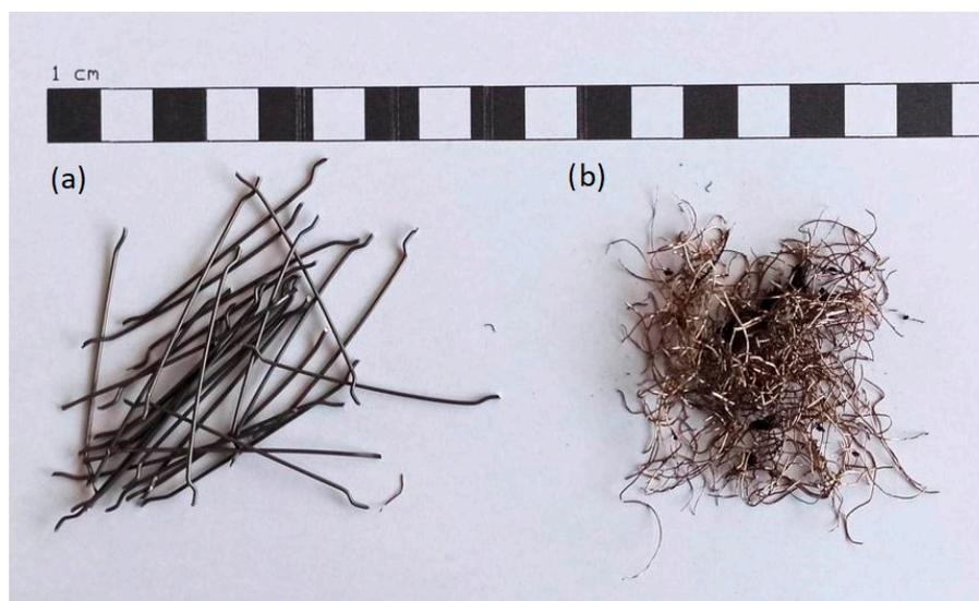
**Figure 2.** (a) Steel hook-end fibers, (b) Steel cord.
