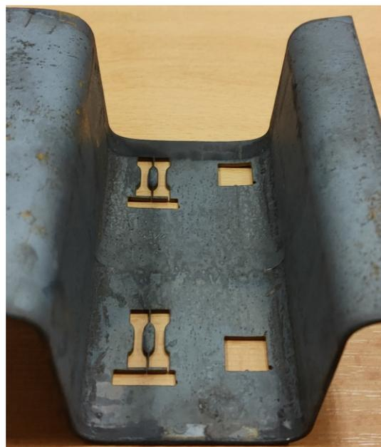
**Figure 8.** Position of mini tensile specimens on the omega profile product from cooled and heated part.
