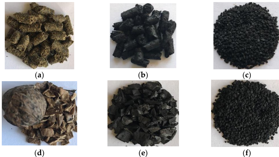
Figure 1. Raw biomass samples: (a)—rapeseed cake; and (d)—walnut shells; Biochars: (b)—rapeseed cake biochar (RSC); (c)—rapeseed cake biochar (RSC) with particles size \leq 1 mm; (e)—walnut shell biochar (WSC); (f)—walnut shell biochar (WSC) with particle size \leq 1 mm.
