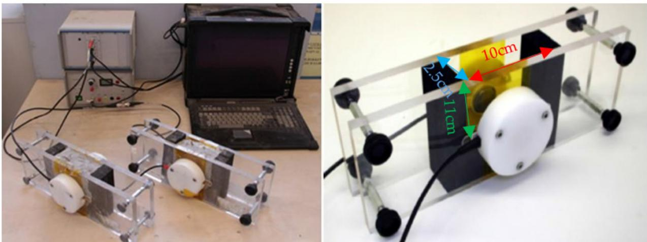
Figure 1. FreshCON system [63] for measuring the ultrasonic pulse velocity.
