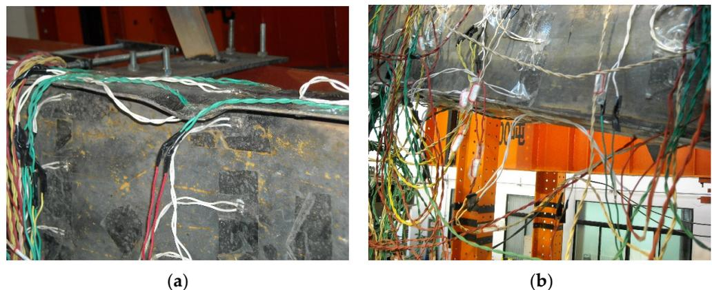
**Figure 8.** Failure phenomenon of specimen SV2. (a) Local buckling of the upper flange; (b) Local buckling of the lower flange.
