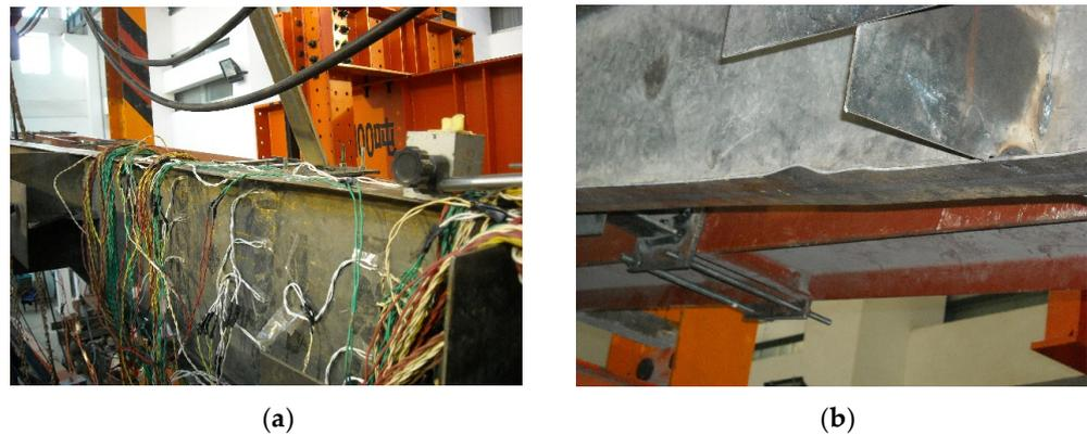
**Figure 7.** Failure phenomenon of specimen SV1. (a) Corrugation on the upper flange of the rafter; (b) Local buckling of the lower flange.
