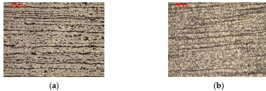
**Figure 3.** Microstructure of base material: (a) delivery state; (b) after long-term exposure at 600 °C, LM-BF.
