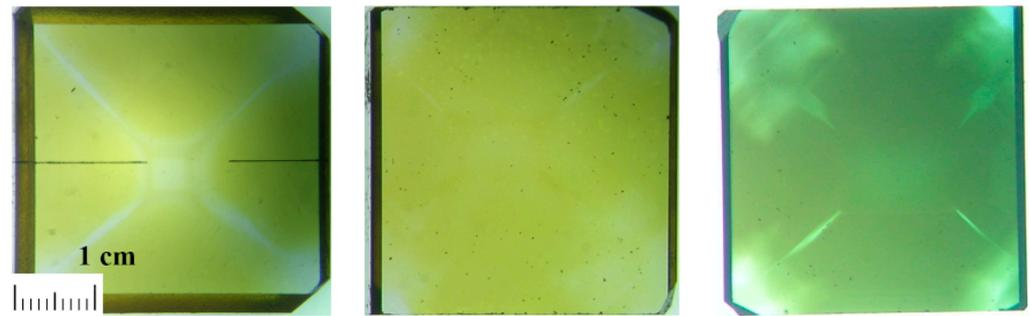
**Figure 5.** Picture of the samples ((left)—reference sample SAFU02, (middle)—sample SAFU01 after electron irradiation (10 MeV,  $1 \times 10^{16}/\text{cm}^2$ ), (right)—sample SAFU01 after electron irradiation (3 MeV,  $1 \times 10^{18}/\text{cm}^2$ )).
