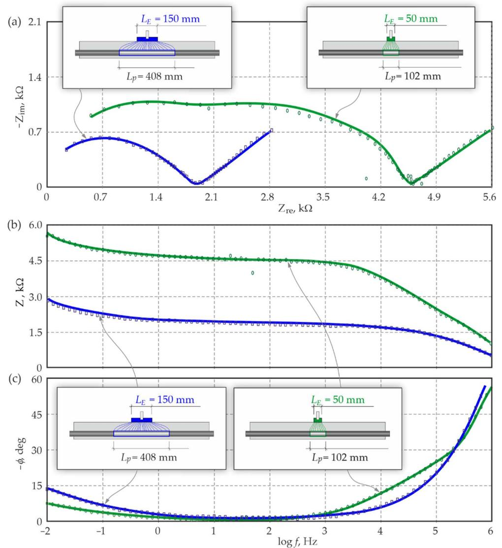
**Figure 9.** Comparative presentation of matching the model spectra (solid lines) to experimental spectra (points) for two lengths  $L_E$  of counter electrodes, according to the original iterative method for determining the polarized area of reinforcement during the EIS tests on reinforced concrete: (a) the Nyquist plot, (b) the Bode  $Z$  ( $\log f$ ) plot, (c) the Bode  $\phi$  ( $\log f$ ) plot.
