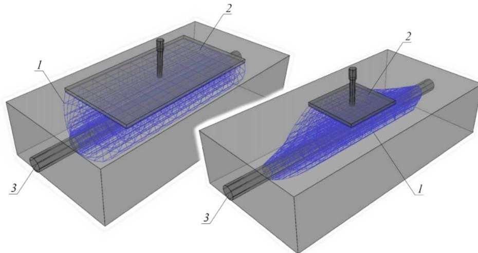
**Figure A2.** Comparison of the “flexible” grid of points representing electrically conductive area of concrete 1 under the alternating current polarization between the counter electrode 2 and the rebar 3; point grids shown in the figure were determined empirically from the Formulas (A1)–(A16).
