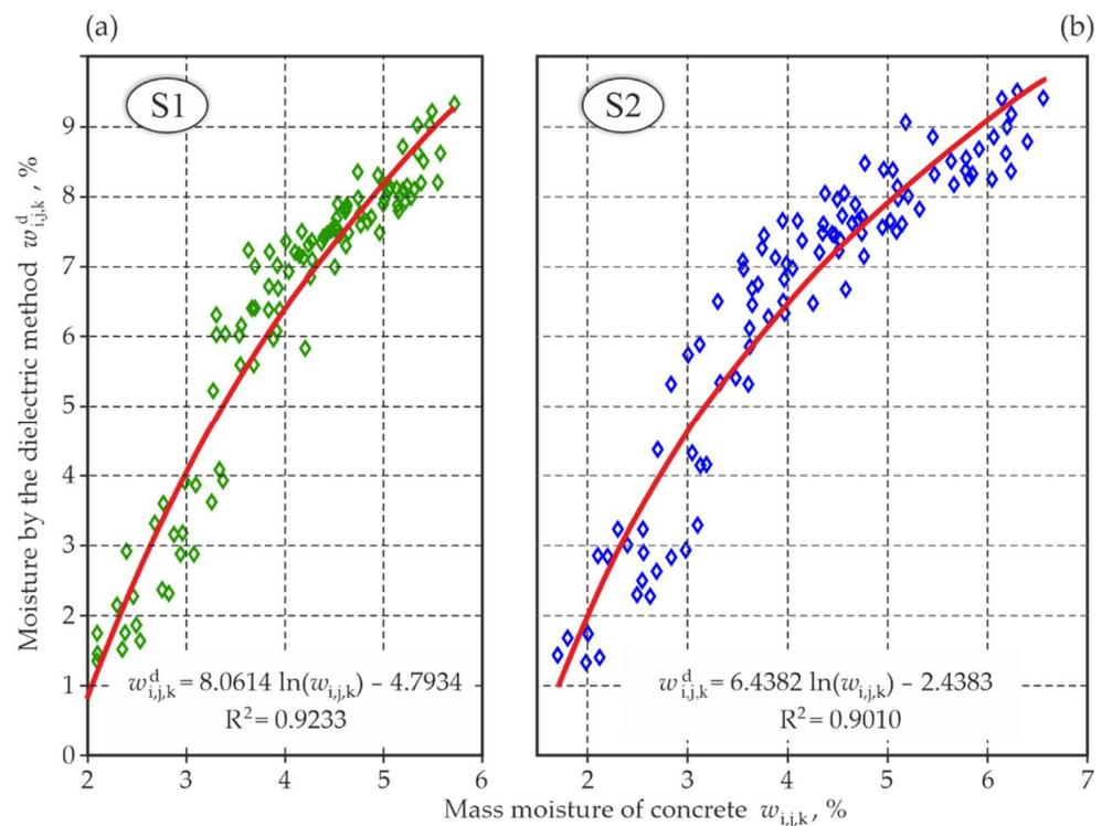
**Figure A3.** Results from correlation tests between the measurements of moisture content by the drying and weighing method and the dielectric method: (a) concrete with the best protective properties—series S1, (b) concrete with chlorides and reduced protective properties—series S2.
