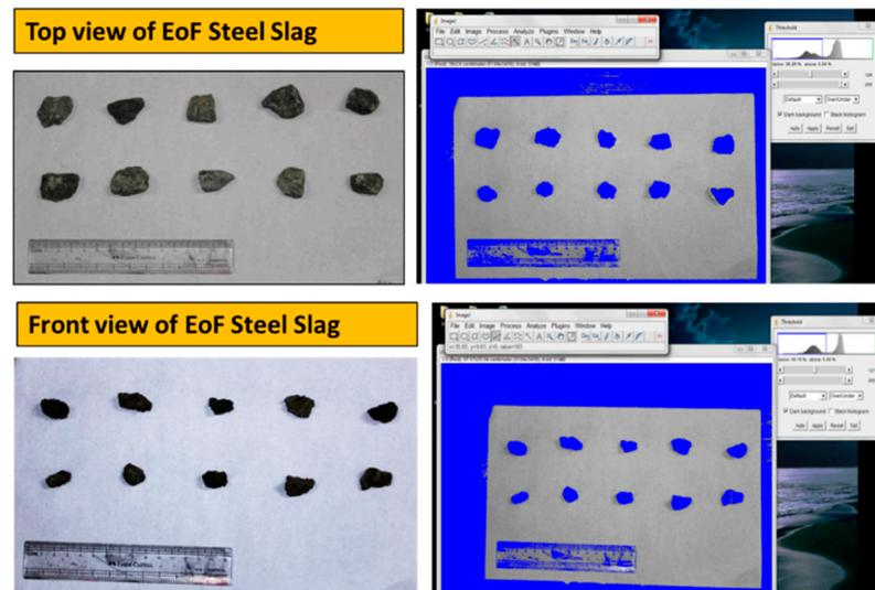
Figure 14. Top and front view of EOF steel slag and thresholded images.
