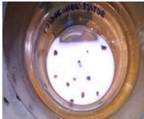
**Figure 4.** Lightweight particles floating in the zinc chloride solution.
