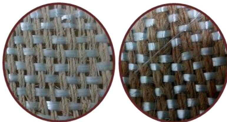
**Figure 7.** Different types of intra-ply hybrid woven natural/glass fiber mats.
