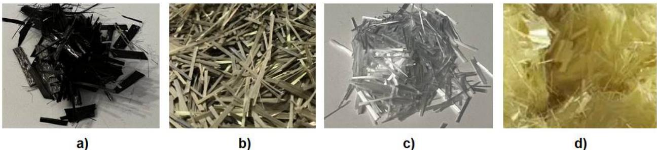
Figure 3. Main type of fibres: (a) carbon fibres; (b) basalt fibres; (c) glass fibres; and (d) aramid fibres.
