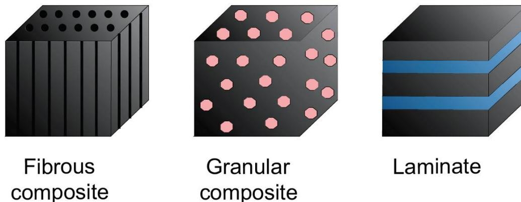
**Figure 1.** Classification of composites regarding their construction, adapted from [11].
