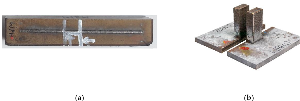
Figure 3. (a) Single-track deposition (b) Multi-track cuboid structure.
