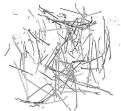
**Figure 20.** 3D computer tomography image with 40 kg/m<sup>3</sup> MSFs.
