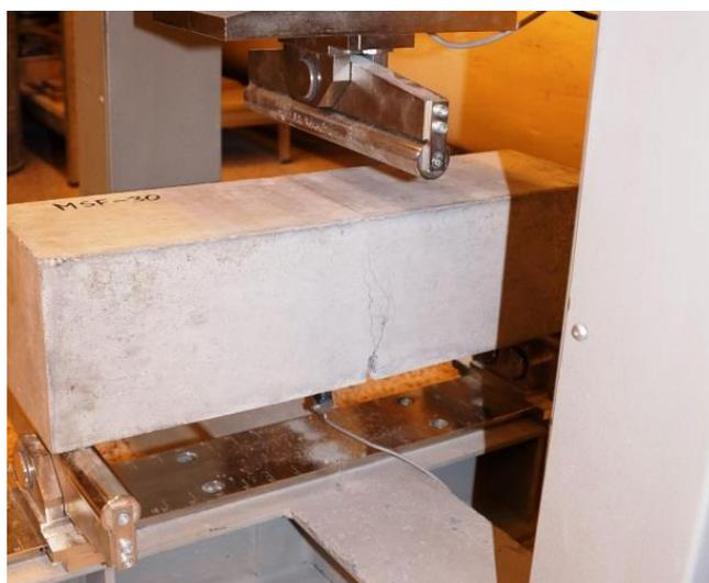
**Figure 3.** Three-point bending of a beam with a notch.
