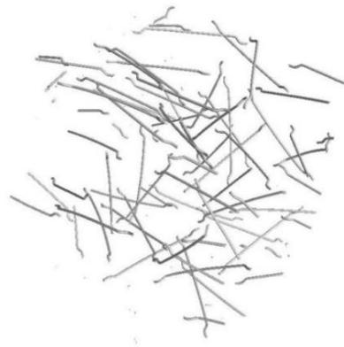
**Figure 18.** 3D computer tomography image with 20 kg/m<sup>3</sup> MSFs.
