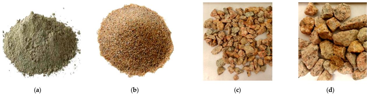
Figure 3. (a) commercial cement, (b) river sand, (c) natural coarse aggregates (NCA)—10 mm, (d) natural coarse aggregates (NCA)—20 mm.
