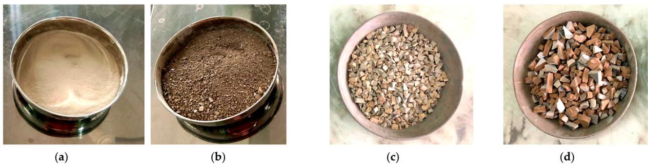
**Figure 4.** (a) waste ceramic cement ( $C_{WC}$ )—75  $\mu\text{m}$ , (b) waste ceramic sand ( $S_{WC}$ )—4.75 mm, (c) waste ceramic aggregate ( $A_{WC}$ )—10 mm, (d) waste ceramic aggregate ( $A_{WC}$ )—20 mm.
