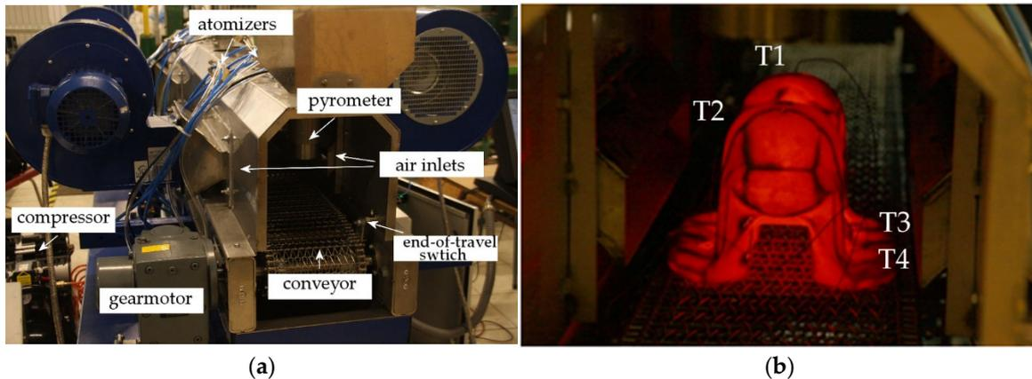
**Figure 2.** Experimental cooling tests: (a) controlled cooling simulator QuenchTube Lab, (b) cooling of the forged sample used for the measurements.
