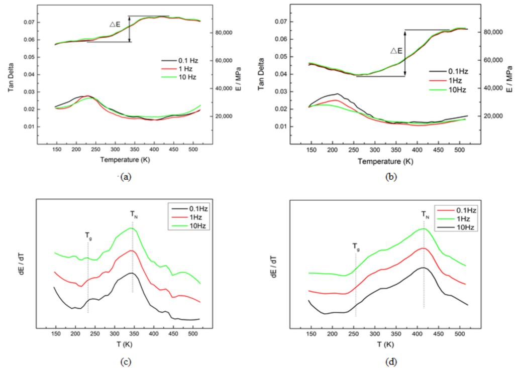
**Figure 2.** Relationship between  $\tan \delta$ , Young's modulus, and temperature of the M2052 alloy (a) as-deposited and (b) after aging. Relationship between  $dE/dT$  and temperature of M2052 alloy (c) as-deposited and (d) after aging.
