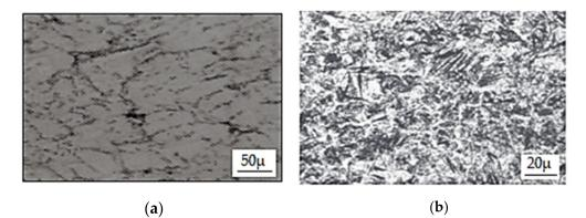
**Figure 10.** Cross-section through a high-speed steel cylinder after a campaign: (**a**) without etching, (**b**) with etching (2% Nital) [38].
