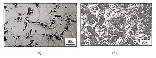
**Figure 9.** Cross-section through a hardened cast iron cylinder after a campaign: (**a**) without etching, (**b**) with etching (2% Nital) [38].
