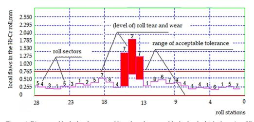
**Figure 4.** Diagram of faults level generated based on the map of faults for the high chromium Hi-Cr cast roll. Source: own, based on [38].
