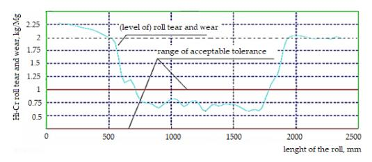
Figure 2. Diagram of high chromium cast rolls local tear and wear levels. Source: own, based on [38].
