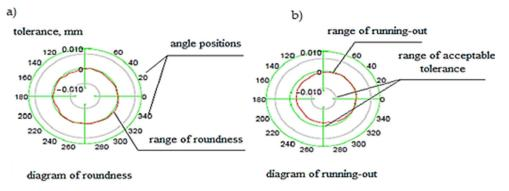
Figure 8. Diagram of defects of rolls made of HSS high-speed steel: (a) out of roundness, (b) run-out. Source: own, based on [38].
