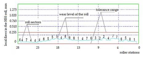
**Figure 7.** Graph-level defects generated on the basis of faults map of type HSS. Source: own, based on [38].
