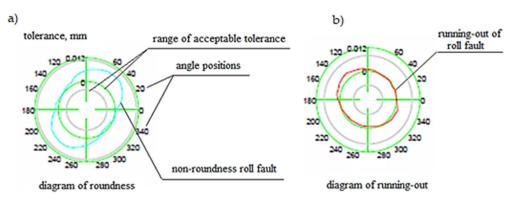
Figure 5. Diagram of defects of rolls made of high chromium cast iron Hi-Cr: (a) irregularities, (b) run-out. Source: own, based on [38].
