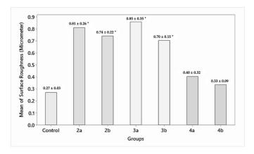
**Figure 4.** Surface roughness (Ra) in  $\mu$ m of the abraded zirconia samples (microns). \* Statistically significant difference between the groups.
