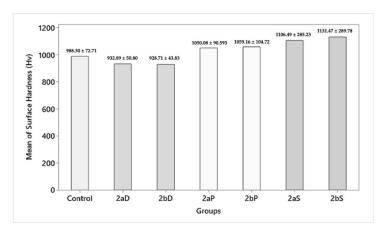
**Figure 9.** Surface hardness after polishing procedures (HV).
