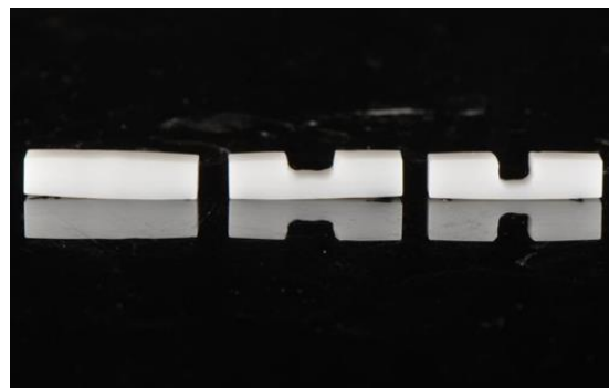
Figure 2. Samples abraded to 1.5 mm and 1 mm residual thickness.
