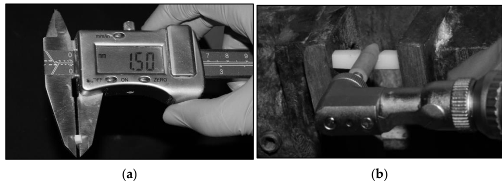
Figure 3. (a) The specimens had dimensions of 15 mm length \times 3 mm width \times 3 mm thickness. The length, width, and thickness were verified with a digital caliper for standardization. (b) Specimens polished using a porcelain polishing kit. Specimens in this group underwent polishing with the commercially available polishing kit (Shofu Porcelain Laminate). Polishing was performed with stroke movements for 30 s by a single trained operator, following the sequence (yellow followed by white polishing points) and speed recommendations (10,000–12,000 rpm) for the system.
