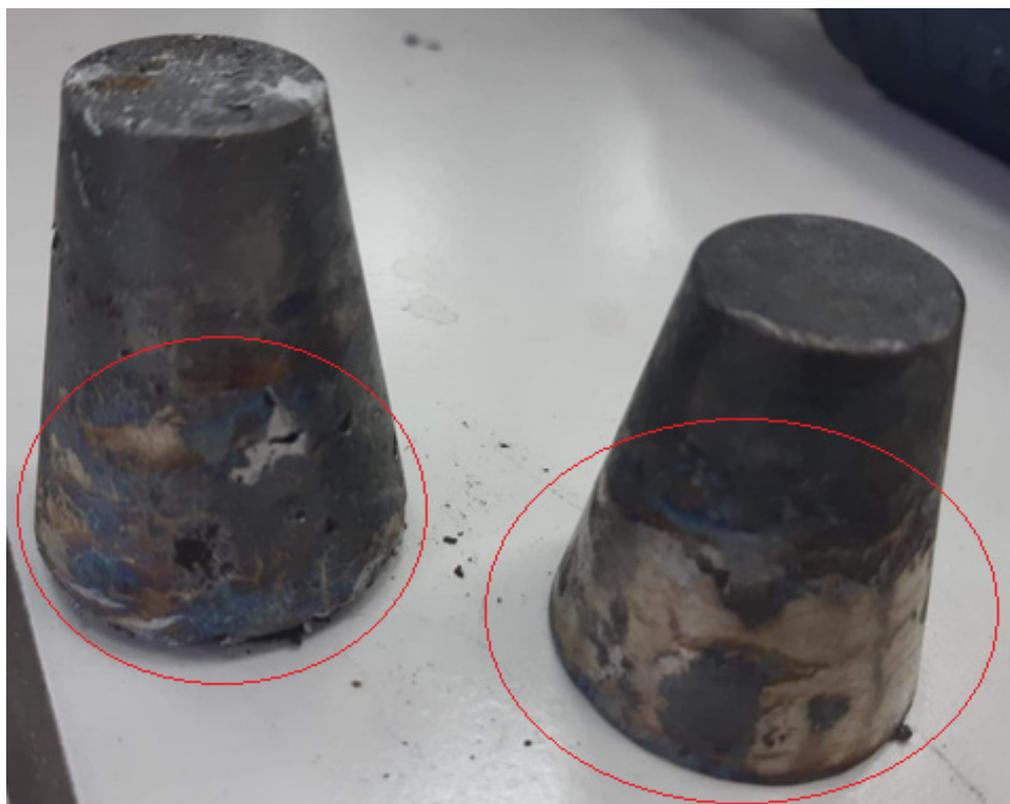
**Figure 5.** Appearances of ingots after pouring molten lead with PCB, red circles show a colorization of ingots.
