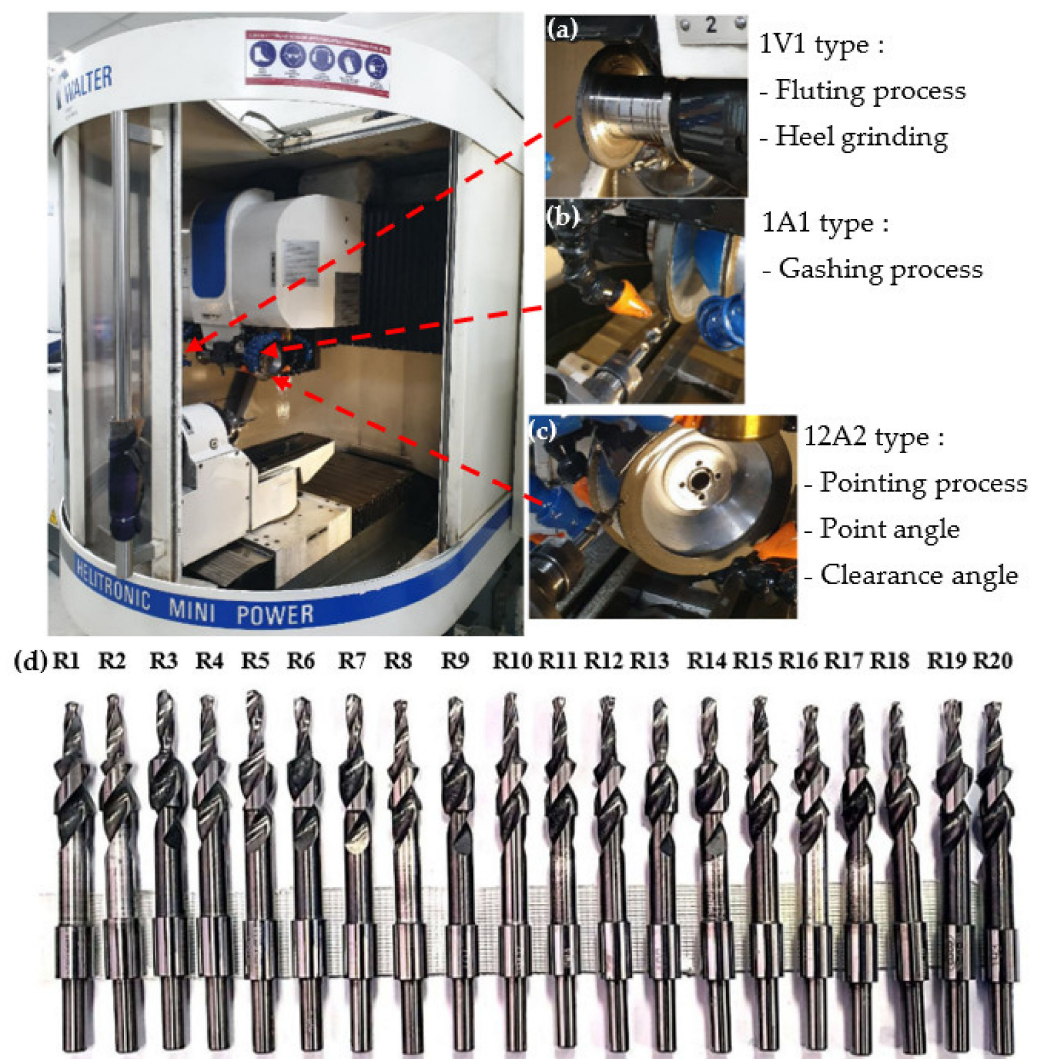
Figure 2. Location of grinding wheel for the tool fabrication (a) fluting wheel, (b) gashing wheel, (c) clearance/point angle wheel, (d) finished drill with customised geometry of twist drill types.
