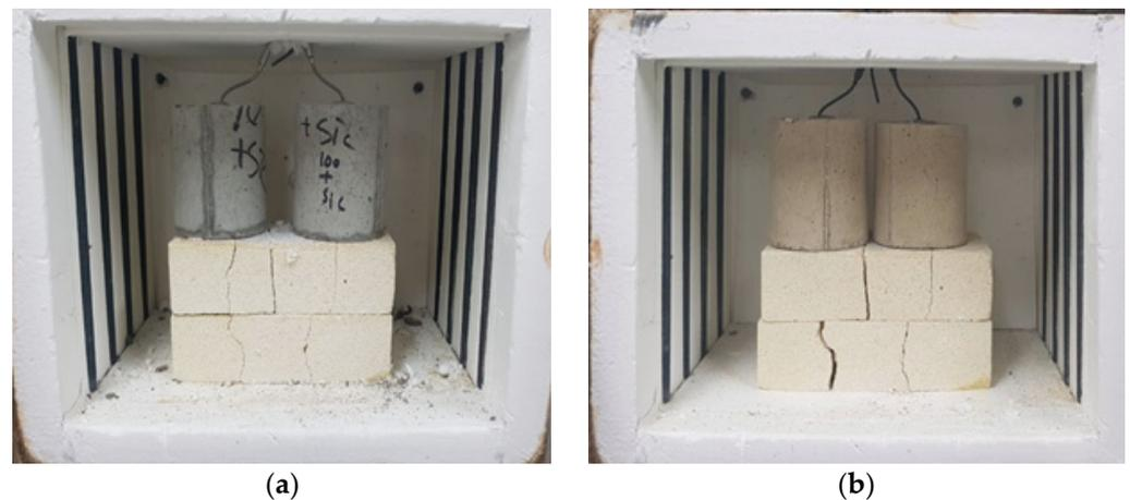
**Figure 2.** Specimens in the electric furnace. (a) before heating at 1000 °C (b) after heating 1000 °C.
