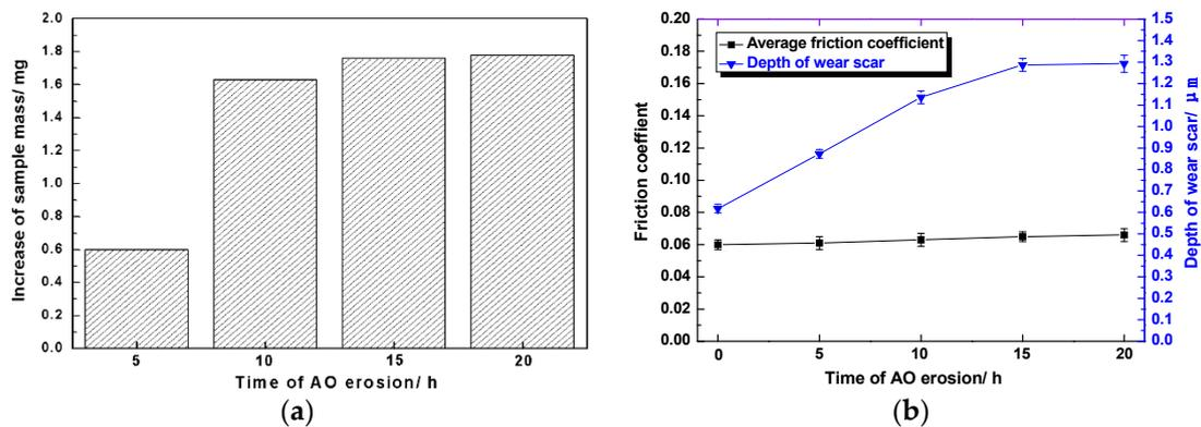
**Figure 6.** The mass and tribological properties of Mo/MoS<sub>2</sub>-Pb-PbS thin film samples after AO treatment at different times: (a) Mass change. (b) Average friction coefficient and variation in wear scar depth.
