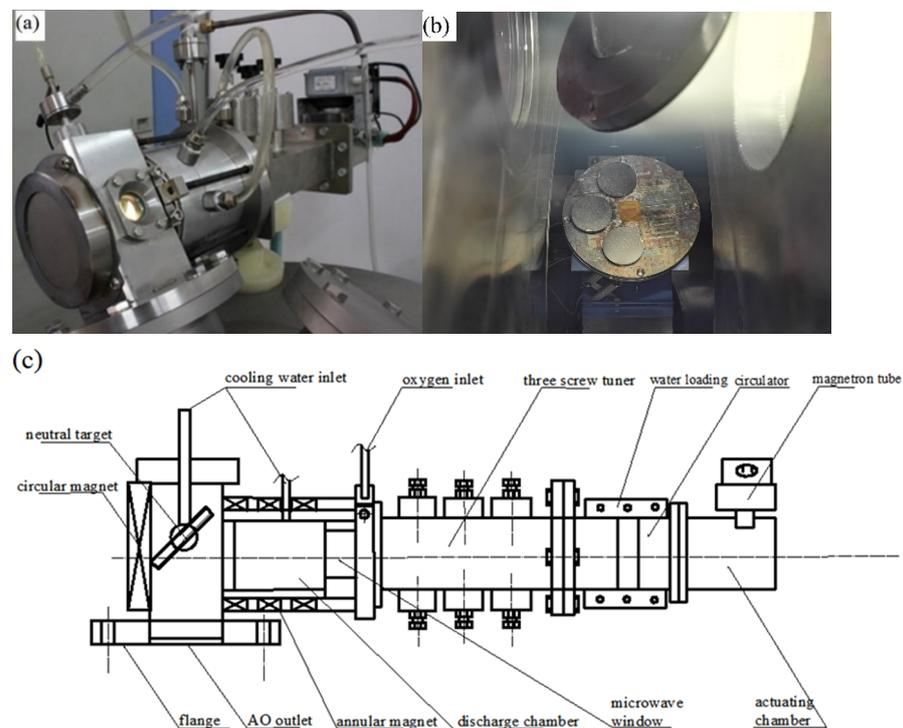
**Figure 1.** (a) AO simulation device, (b) picture of samples exposing by AO, (c) structure schematic of AO emission device.
