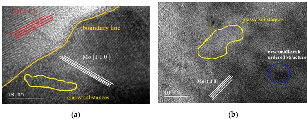
**Figure 3.** TEM images of Mo/MoS<sub>2</sub>-Pb-PbS composite film before and after AO erosion: (a) composite film without AO erosion, (b) composite film with AO erosion.
