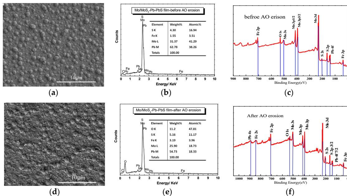
**Figure 2.** SEM morphology, EDS composition, and XPS survey of Mo/MoS<sub>2</sub>-Pb-PbS composite film before and after AO erosion: (a–c) without AO erosion. (d–f) AO erosion.
