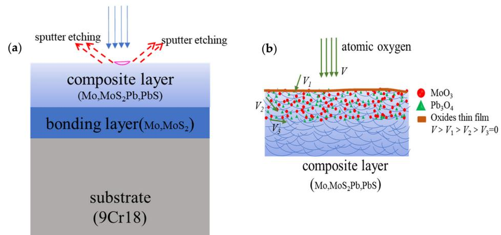
**Figure 7.** Schematic of AO etching and oxidation: (a) Schematic diagram of sputter-etching; (b) Diagram of oxidation.
