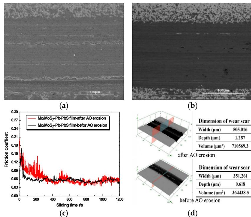
**Figure 5.** Comparison of tribological properties of Mo/MoS<sub>2</sub>-Pb-PbS composite film before and after AO treatment: (a) The wear scar morphology before AO erosion. (b) The wear scar morphology after AO erosion. (c) Friction coefficient curve. (d) 3D wear scar morphology.
