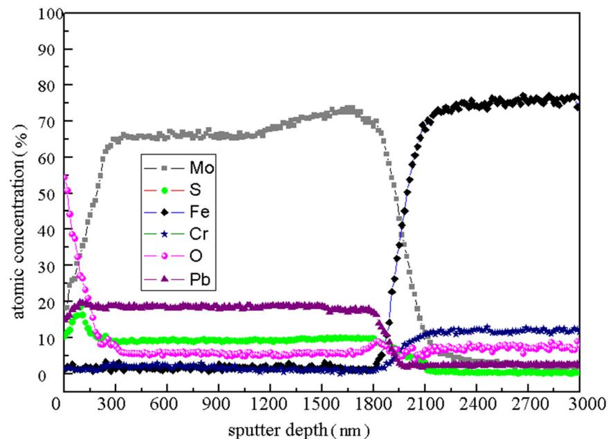
**Figure 4.** AES Etching Test Results of Mo/MoS<sub>2</sub>-Pb-PbS Film in Depth Direction after AO Erosion.
