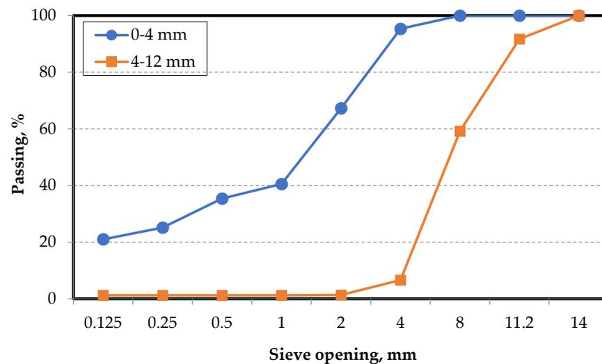
Figure 3. Particle size distribution of the aggregates.
