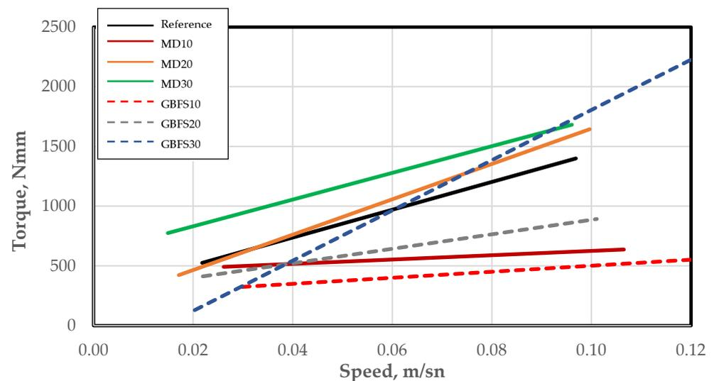
**Figure 5.** Rheometer analyses of the SCC mixtures.
