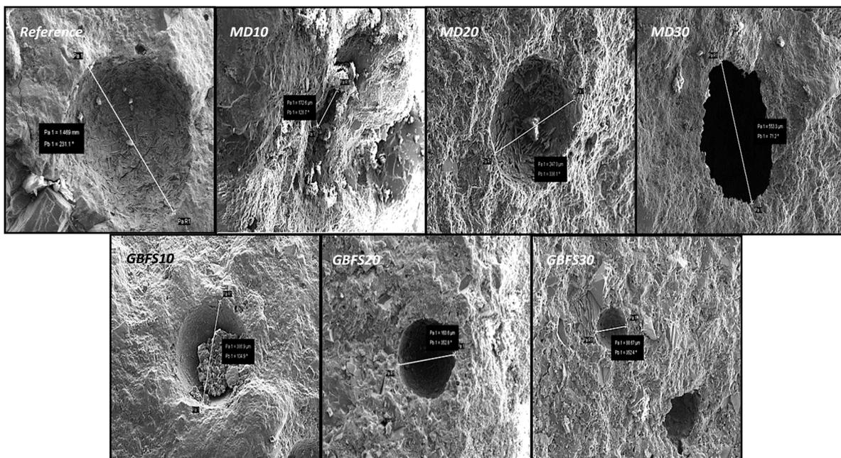
Figure 10. The pore structure of the SCC mixtures.
