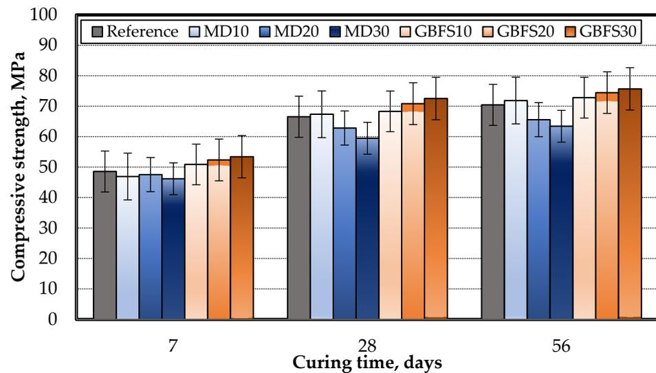
**Figure 6.** Compressive strength of the SCC specimens.
