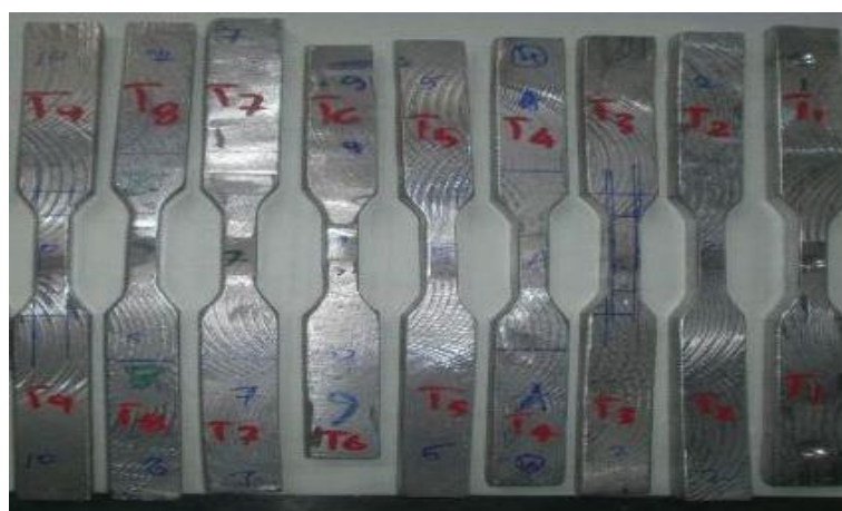
Figure 2. Tensile test samples as per ASTM Standards.
