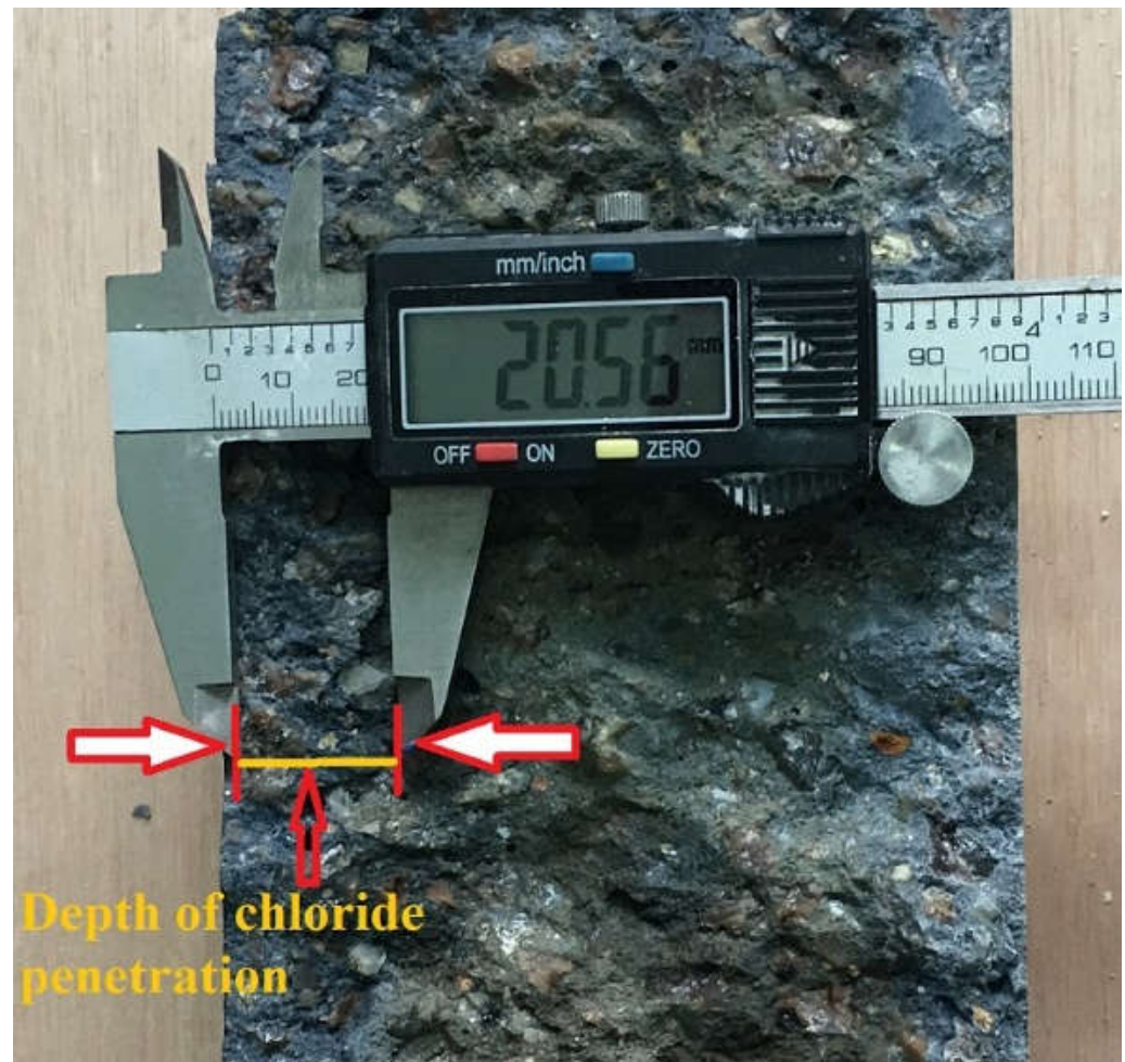
Figure 3. Depth of chloride penetration after spraying with \text{AgNO}_3 solution.
