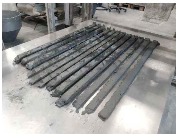
Figure 13. Filaments printed with SHCC mixtures Ref and SE-CE; photo was taken the day after printing and following removal of the cover foil.
