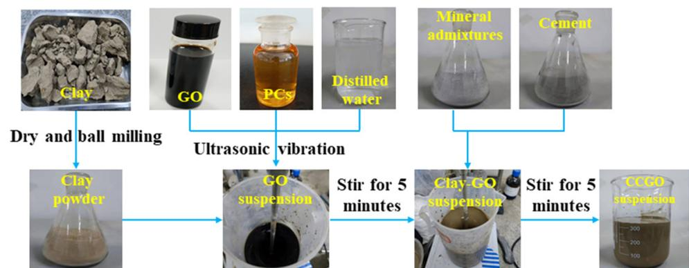
**Figure 1.** Preparation process of clay–cement–graphene oxide (CCGO) grouting materials.
