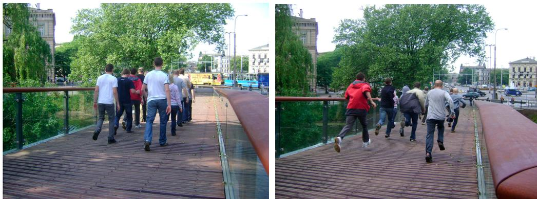
Figure 22. Examples of the dynamic tests carried out on the footbridge in Wrocław (synchronized walking and running).
