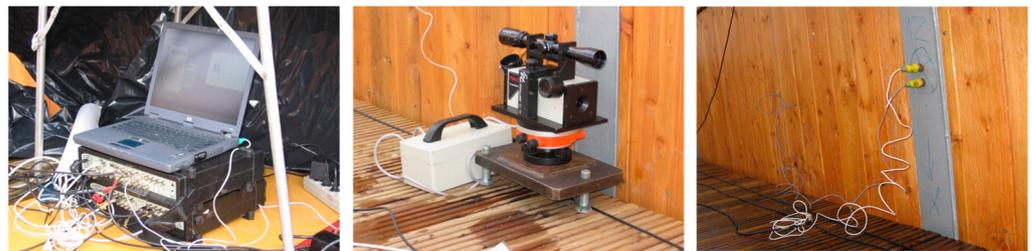
**Figure 8.** Measurement devices (Bruel & Kjaer amplifiers, Noptel OY PSM200 laser device and Endevco accelerometers).
