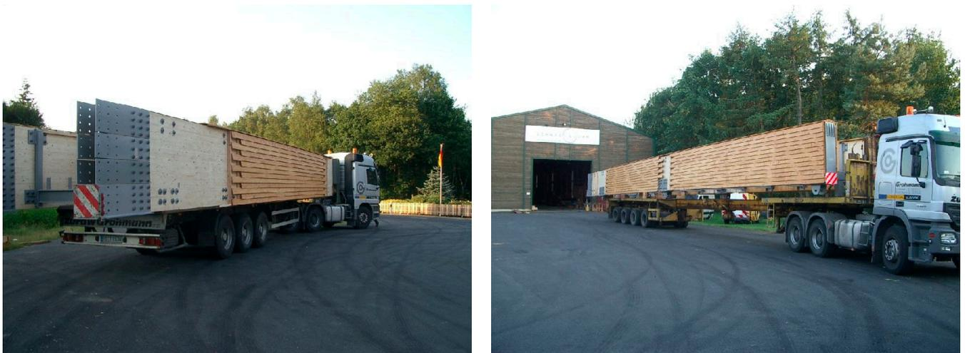
Figure 4. Assembling segments of the deck during their transport on the specialized lorries from the woodworking company in Germany to the construction site in Poland (Photos credit: Schmees & Lühn Holz- und Stahlgenieurbau GmbH & Co. KG and Mosty-Wroclaw Design & Research Office).
