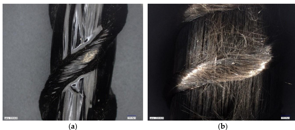
Figure 6. Magnified images of HFRP bars (20 × 20): (a) before testing; (b) after testing.
