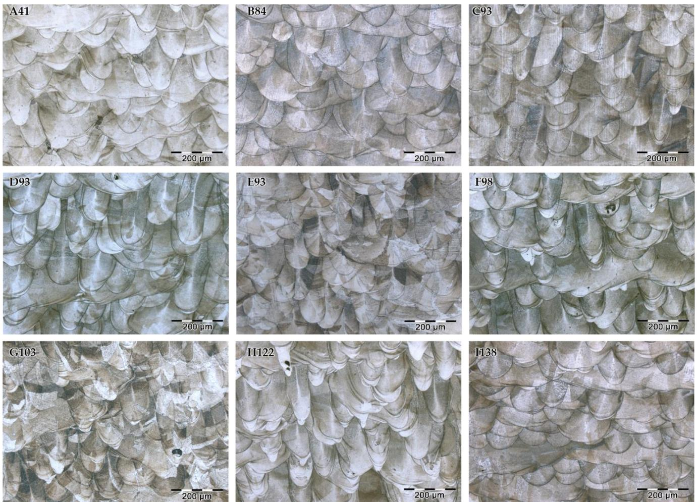
**Figure 3.** Optical micrographs of the cross section (XZ plane) of SLM samples after etching.
