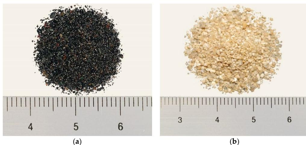
**Figure 1.** Photograph of fine aggregates used. (a) Magnetite fine aggregate. (b) River sands.
