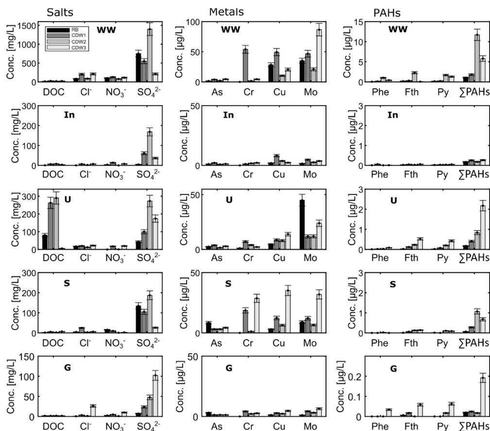
**Figure 3.** Concentrations of salts, metals and PAHs from short column tests at L/S 2 ratio of railway ballast (RB) and three sets of construction and demolition waste (CDW); WW represents concentrations in the washing water used for cleaning and separation of the input material (In) into the different size fractions silt (U), sand (S) and gravel (G). Error bars represent uncertainties in measurements.
