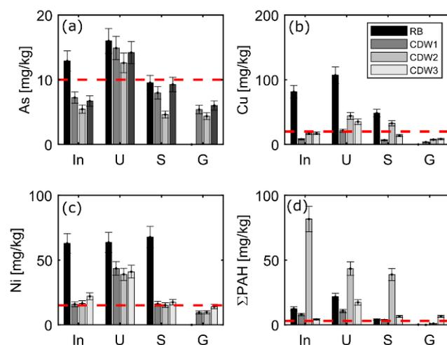
**Figure 2.** Concentrations of (a) As, (b) Cu, (c) Ni, and (d) the sum of the 16PAHs in solids: Input material (In), silt (U), sand (S) and gravel (G) of railway ballast (RB) and three sets of construction and demolition waste (CDW); input represents the material prior to separation into the different fractions (silt, sand and gravel), and the red dashed lines indicate precautionary values for sandy soils [19]. Error bars represent uncertainties in measurements.
