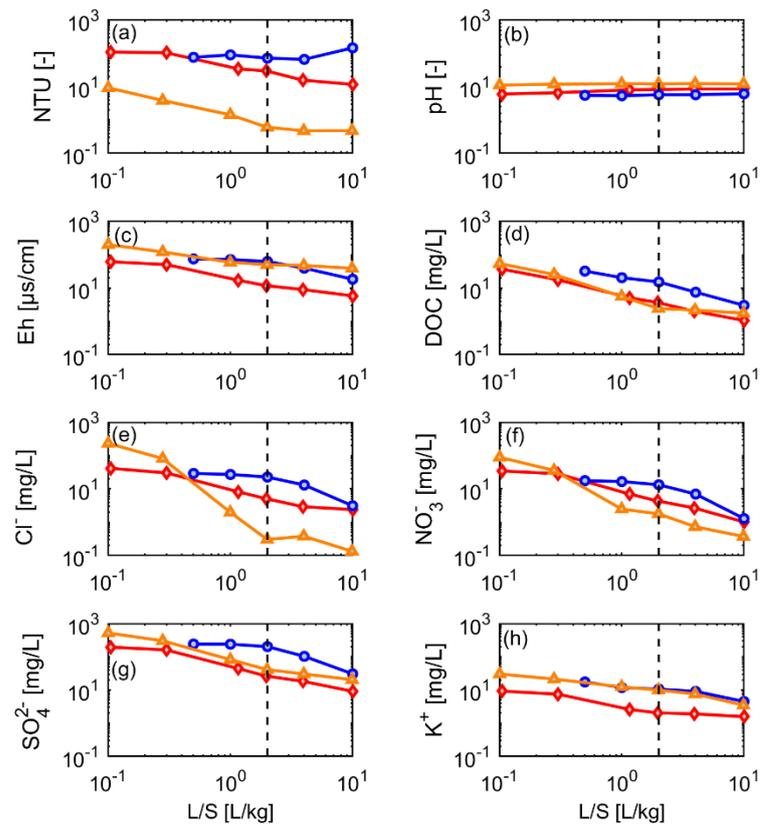
**Figure 6.** Leaching behavior of selected “salts” from different grain-size fractions of CDW material (CDW3) until a liquid-to-solid (L/S) ratio of 10 (dotted line  $L/S = 2$ ); red diamonds: input material (mixture), blue circles: silt ( $<0.063$  mm), orange triangles: sand (0–0.2 mm). (a) TSS, (b) pH, (c) Eh, (d) DOC, (e)  $Cl^-$ , (f)  $NO_3^-$ , (g)  $SO_4^{2-}$ , and (h)  $K^+$ .
