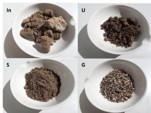
**Figure 1.** Solid waste fractions of construction and demolition waste (CDW3) as received from the recycling plant: input material (In) as well as silt (U), sand (S) and gravel (G) fractions obtained after wet-treatment.
