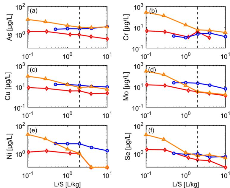
**Figure 7.** Leaching behavior of selected metals from different grain size fractions of CDW material (CDW3) until a liquid-to-solid (L/S) ratio of 10 (dotted line  $L/S = 2$ ); red diamonds: input material (mixture), blue circles: silt ( $<0.063$  mm), orange triangles: sand (0–0.2 mm). (a) As, (b) Cr, (c) Cu, (d) Mo, (e) Ni, and (f) Se.
