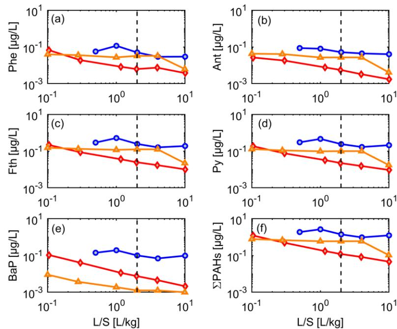
**Figure 8.** Leaching behavior of selected PAHs from different grain-size fractions of CDW material (CDW3) until a liquid-to-solid (L/S) ratio of 10 (dotted line L/S = 2); red diamonds: input material (mixture), blue circles: silt (<0.063 mm), orange triangles: sand (0–0.2 mm). (a) Phe, (b) Ant, (c) Fth, (d) Py, (e) BaP, and (f) the sum of 16PAHs.
