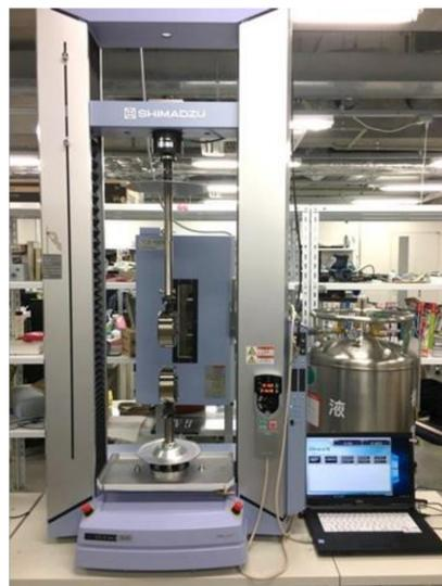
**Figure 4.** Universal mechanical testing machine (AG-X plus, SHIMADZU Co., Ltd., Kyoto, Japan) for conducting tensile tests.
