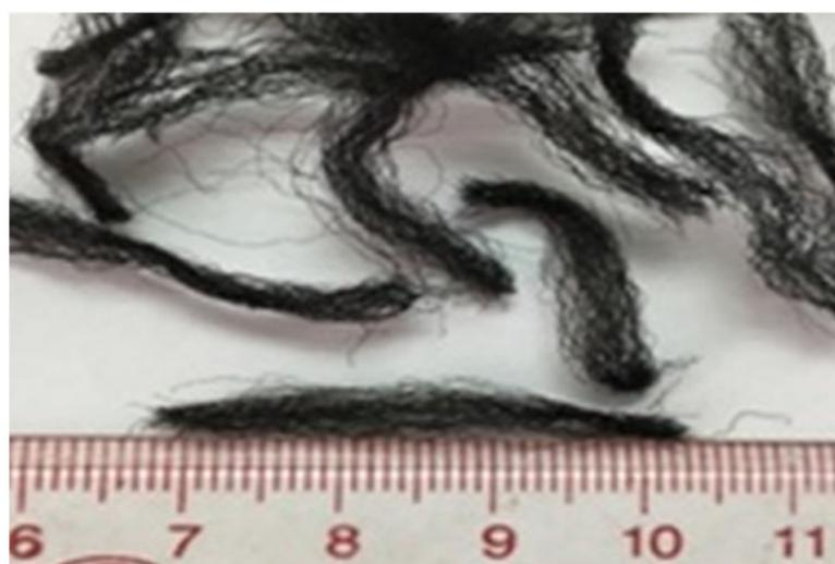
**Figure 1.** Size and shape of PP fibers used.
