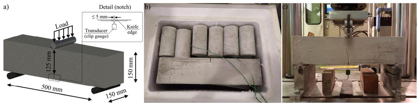
**Figure 2.** (a) 3PBT setup; (b) freezing procedure and temperature monitoring; (c) 3PBT at  $-30\text{ }^{\circ}\text{C}$ .
