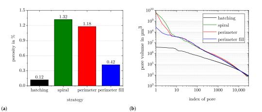
**Figure 7.**  $\mu$ CT analysis of samples fabricated with different strategies. (**a**): Porosity values measured with  $\mu$ CT. (**b**): Pores sorted by size in descending order. The spiral and perimeter strategies lead to similar distributions, while the perimeter fill strategy can reduce the size of the few largest pores. The hatching strategy results in smaller pores overall.
