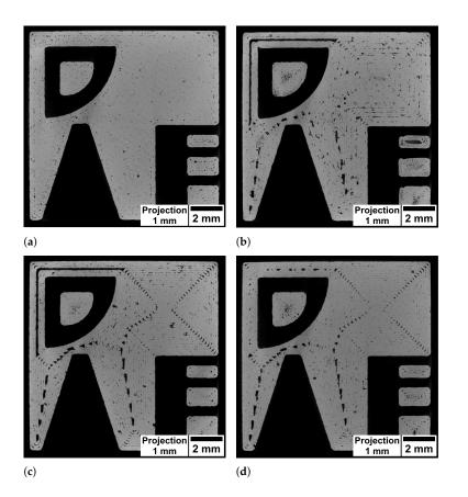
**Figure 5.** Projection images of 1 mm depth of specimens built with different strategies. (**a**): hatching strategy, (**b**): spiral strategy, (**c**): perimeter strategy, (**d**): perimeter fill strategy.
