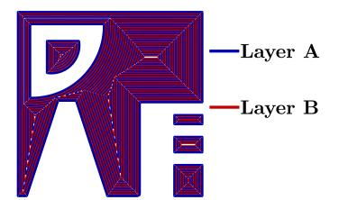
**Figure A2.** Two layers of proposed improved perimeter strategy. The first layer is shown red, while the next layer is shown blue. The first line distance is reduced to  $75 \,\mu\text{m}$  in the blue layer to place scan lines between the scan lines of the red layer to avoid lack of fusion pores between paths.
