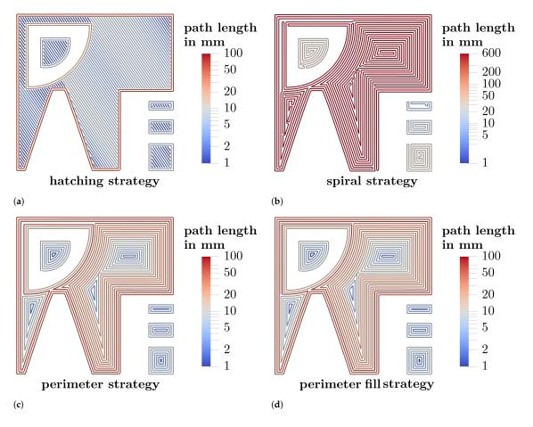
**Figure 3.** Exemplary layer views of different scan strategies. The paths are color coded according to the respective path lengths. (a): hatching strategy, (b): spiral strategy, (c): perimeter strategy, (d): perimeter fill strategy.
