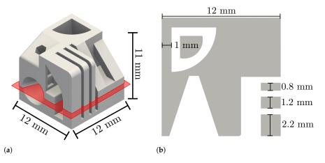
**Figure 1.** Geometry used in this investigation. (**a**): 3D rendering of the geometry. The layer highlighted in red will be investigated in detail. (**b**): Cross section of the layer highlighted red.
