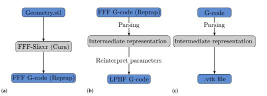
**Figure 2.** Schematic of build job generation and analysis. (a): FFF job generation. (b): Conversion to LPBF build job. (c): Conversion of build job to visualisation file for further 3D covisualisation with  $\mu$ CT data.
